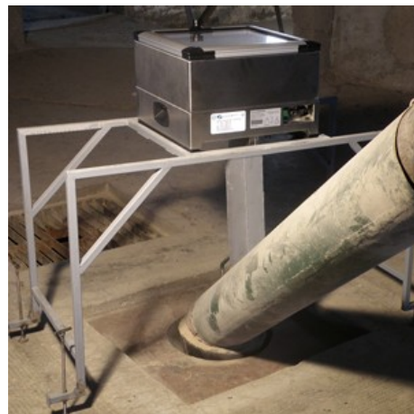
Figure 3. Display of pedestal and tube plug for setting of dispenser on tube for insertion grain.
