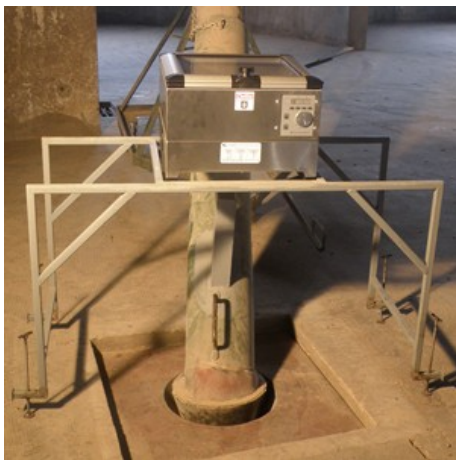
Figure 2. Dispenser is set by the pedestal on tube for insertion grain, on which was built-in tube plug for connection with a dispensers telescope.
