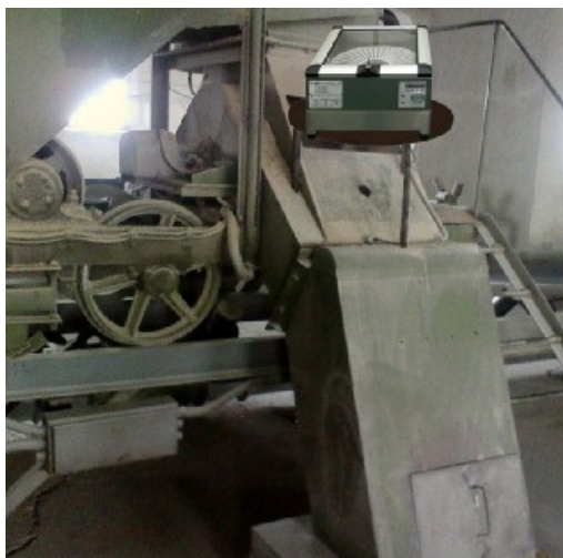
Figure 4. Dispenser is on top of the channel of the filling tube with trolley for filling in cells with grain, and sensor may be placed into the pipe opening under the dispenser.
