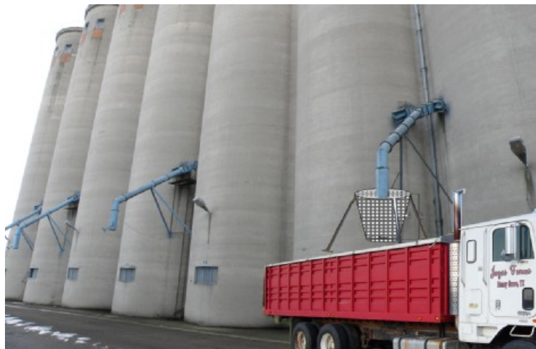
Figure 11. By gravitation emptying of a silo cell, grainy goods pass through the set grid while Detia bags remain in the grid, and are removed after loading of a vehicle – vessel.
